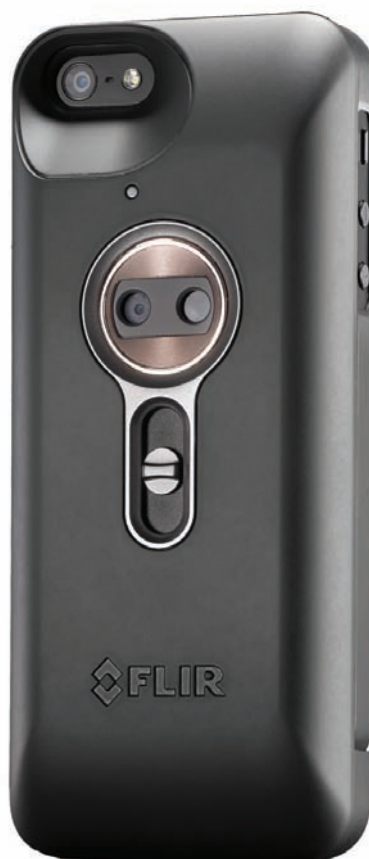
The Flir One unit fits onto a standard current-generation iPhone.
