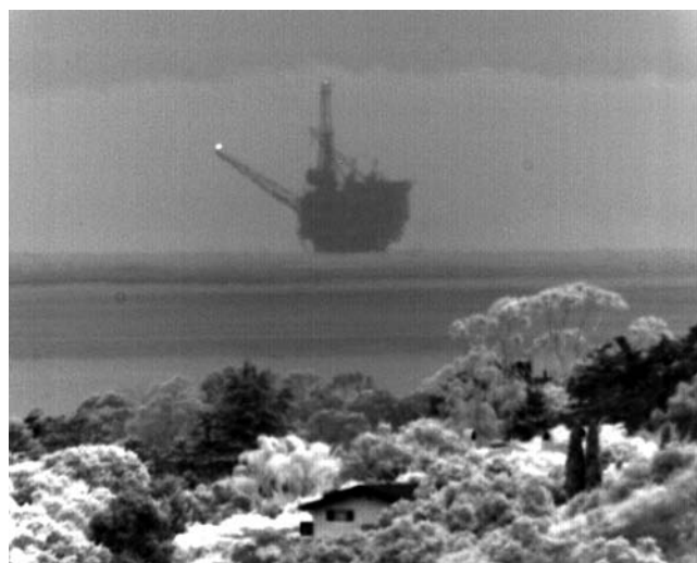
Figure 4. In this visible-light image (left) of an oil rig at a 47-km range, the oil rig can barely be seen, but it is visible in the SWIR image (right), which was taken at the same distance.
