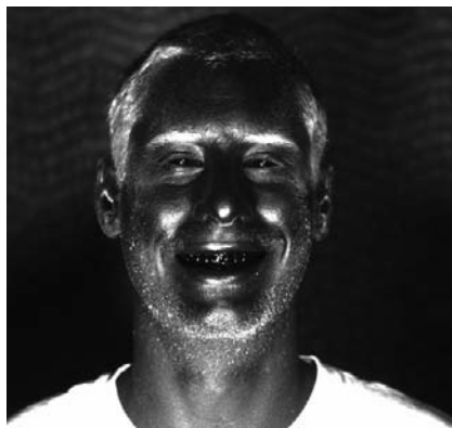
Figure 3. A SWIR image of a man (2 to 2.5 \mu\text{m} ) with light skin color. Water just below the skin's surface absorbs SWIR radiation in this band very well.
