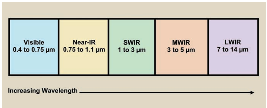
Figure 1. The visible and infrared spectrum can be broken down into subbands. IR imaging technology covers a range of the spectrum, and images vary with the waveband. Images courtesy of Flir Commercial Systems.
