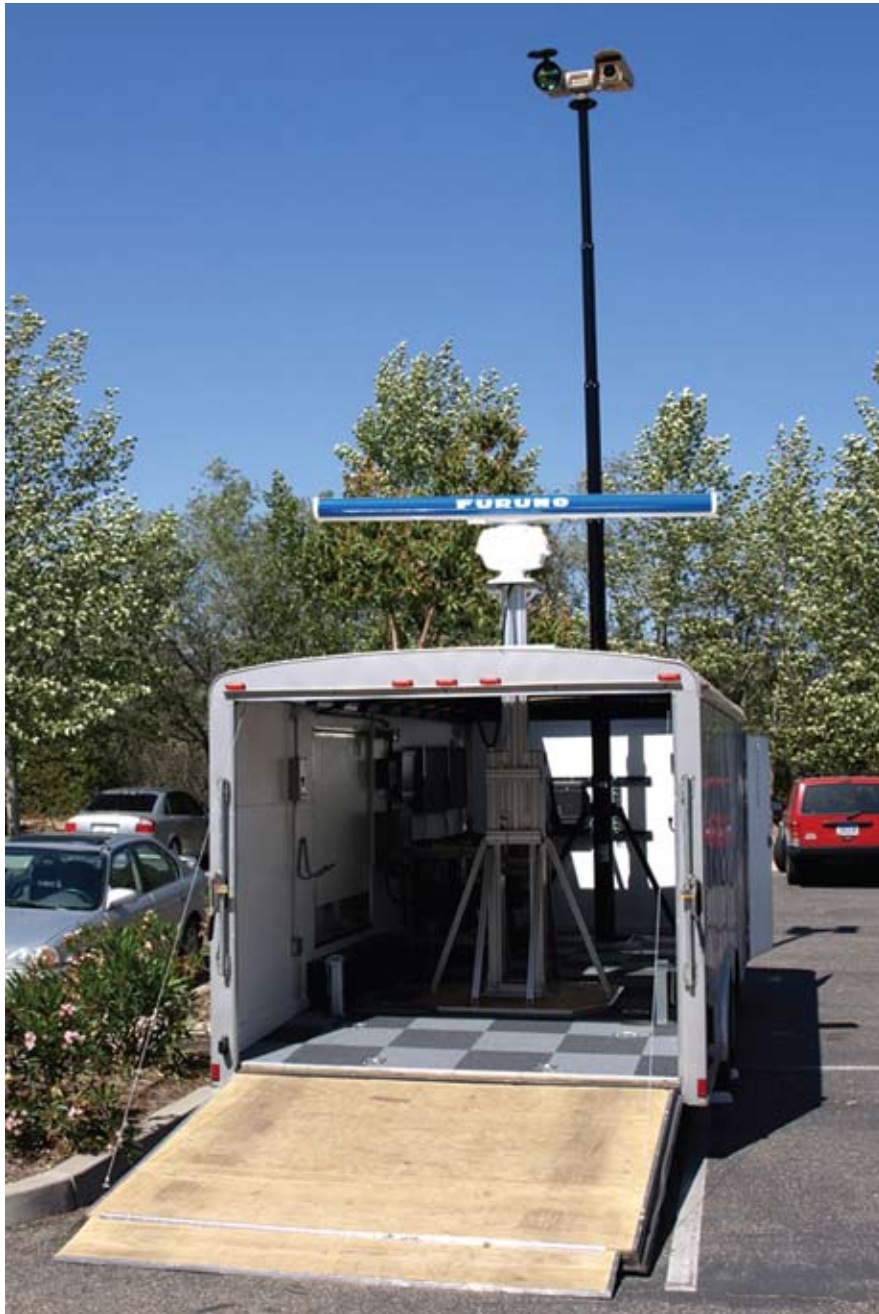
Figure 3a: A FLIR CVS radar trailer.
