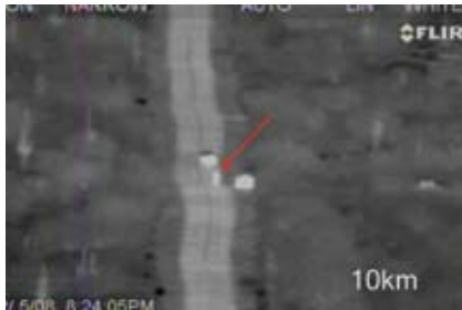
Figure 2b: a midwave IR image of man and two cars at 10km range with 2X digital zoom. The red arrow points to the man.
