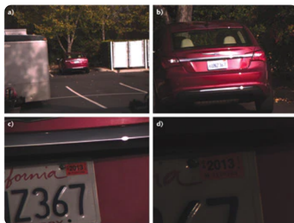
FIGURE 4. Loss of light is obvious when zooming from 135 mm focal length (a) to 500 mm (b), 1000 mm (c), and 2000 mm (d; nearly black). All variables except for f/\# due to focal length change were held constant.
