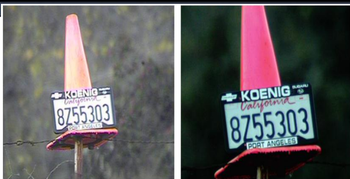
Figure 10a. Left: Hitachi, Right Tau CNV, 4:46PM, 6 minutes before sunset. 300 Lux. Both Lenses' irises probably closed down to f/16 by cameras' auto iris circuits.
