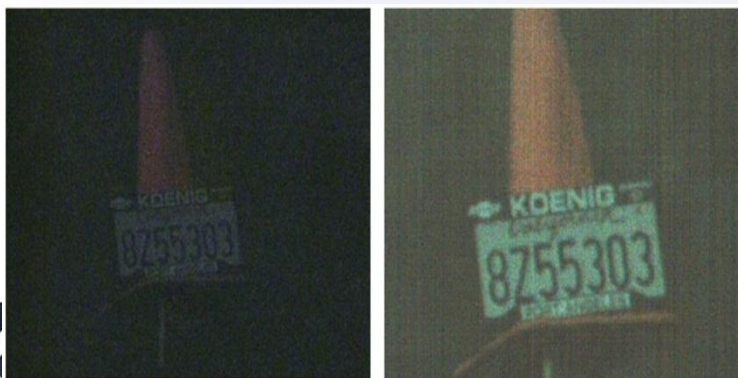
Figure 10e. Left: Hitachi, Right Tau CNV, 5:26 PM, 34 minutes after sunset. 0.2 Lux. Contrast is dropping rapidly with time.
