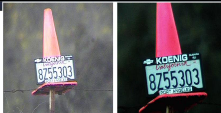
Figure 10b. Left: Hitachi, Right Tau CNV, 4:56PM, 4 minutes after sunset. 97 Lux. Note that the background has gone out of focus. This is because the lens iris has fully dilated and the f/number has decreased from f/16 to f/3.5.
