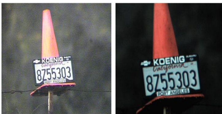
Figure 10c. Left: Hitachi, Right Tau CNV, 5:11 PM, 19 minutes after sunset. 5 Lux. More detail is showing on the orange cone surface in the Tau CNV image compared to earlier Tau CNV images. The cameras' exposures are starting to drop and fixed-pattern noise is apparent in the Hitachi image.
