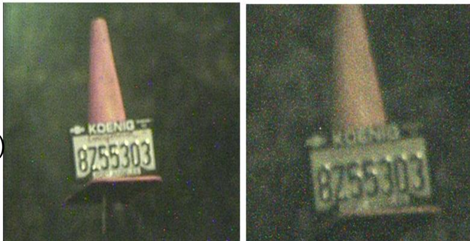
Figure 10h. Left: Hitachi, Right: Tau CNV, 5:49 PM, 57 minutes after sunset. 0.013 Lux . Both cameras have been set for 1Hz frame rate operation. The Tau CNV integration time is 966 msec and the Hitachi has Sens Up set to "Autox32", which means that up to 32 frames can be summed as needed.
