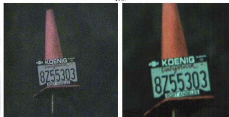
Figure 10b. Left: Hitachi, Right Tau CNV, 4:56PM, 4 minutes after sunset. 97 Lux. Note that the background has gone out of focus. This is because the lens iris has fully dilated and the f/number has decreased from f/16 to f/3.5.
