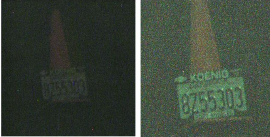
Figure 10h. Left: Hitachi, Right: Tau CNV, 5:49 PM, 57 minutes after sunset. 0.013 Lux . Both cameras have been set for 1Hz frame rate operation. The Tau CNV integration time is 966 msec and the Hitachi has Sens Up set to "Autox32", which means that up to 32 frames can be summed as needed.
