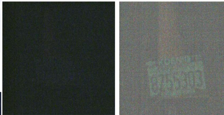
Figure 10f. Left: Hitachi, Right: Tau CNV, 5:32 PM, 40 minutes after sunset. 0.060 Lux. The Hitachi image is dark and the license number is no longer legible.
